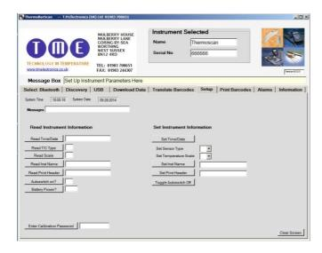
Once you have set your parameters, you can check that the settings have been stored by using the *Read* functions. The instrument is now ready for use.
