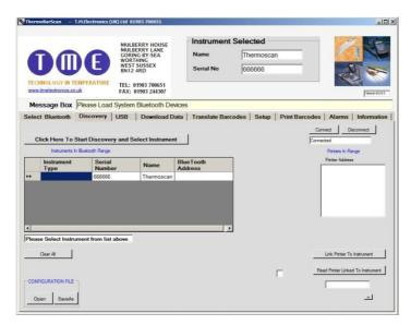
The devices within Bluetooth range will be displayed and their Bluetooth addresses shown. Click to connect to the instrument you wish to connect to.
