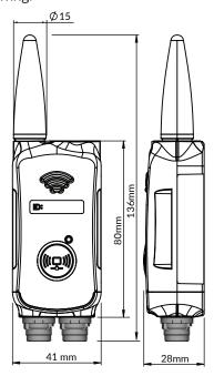
Designed to work with tek troniks D3 868Mhz wireless base stations and is compatible with a full range of tek troniks intelligent sensors.
