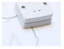
Attach the probe sensor to the object you wish to monitor using a TAPS adhesive pad or similar tape. Run the probe wire back to the TC Wall Port and fix the back panel to the wall using the slotted screw holes provided.
